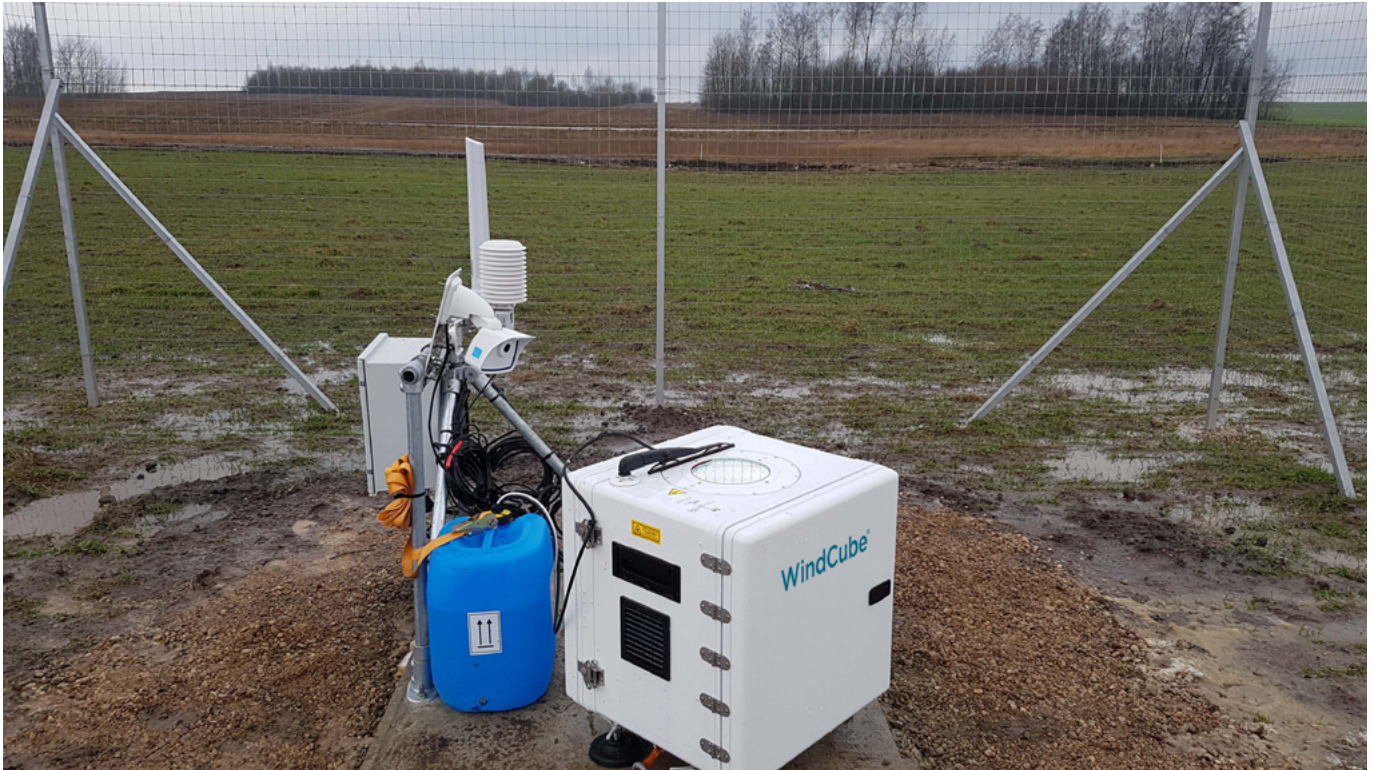
Figure 7: WindCube deployment in greenfield area for Wind Resource Assessment (WRA) — Example deployment in greenfield area in Lithuania. The space around the lidar is secured with a fence; the water tank and lidar are fixed to the ground. Photo courtesy of Kjeller Vindteknikk.
