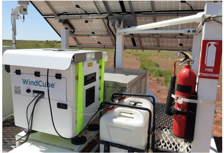
Figure 15: Sunshade atop of WindCube unit installed on a trailer in the desert — Sunshade and trailer installations reduce the exposure of the lidar to direct solar radiation.
