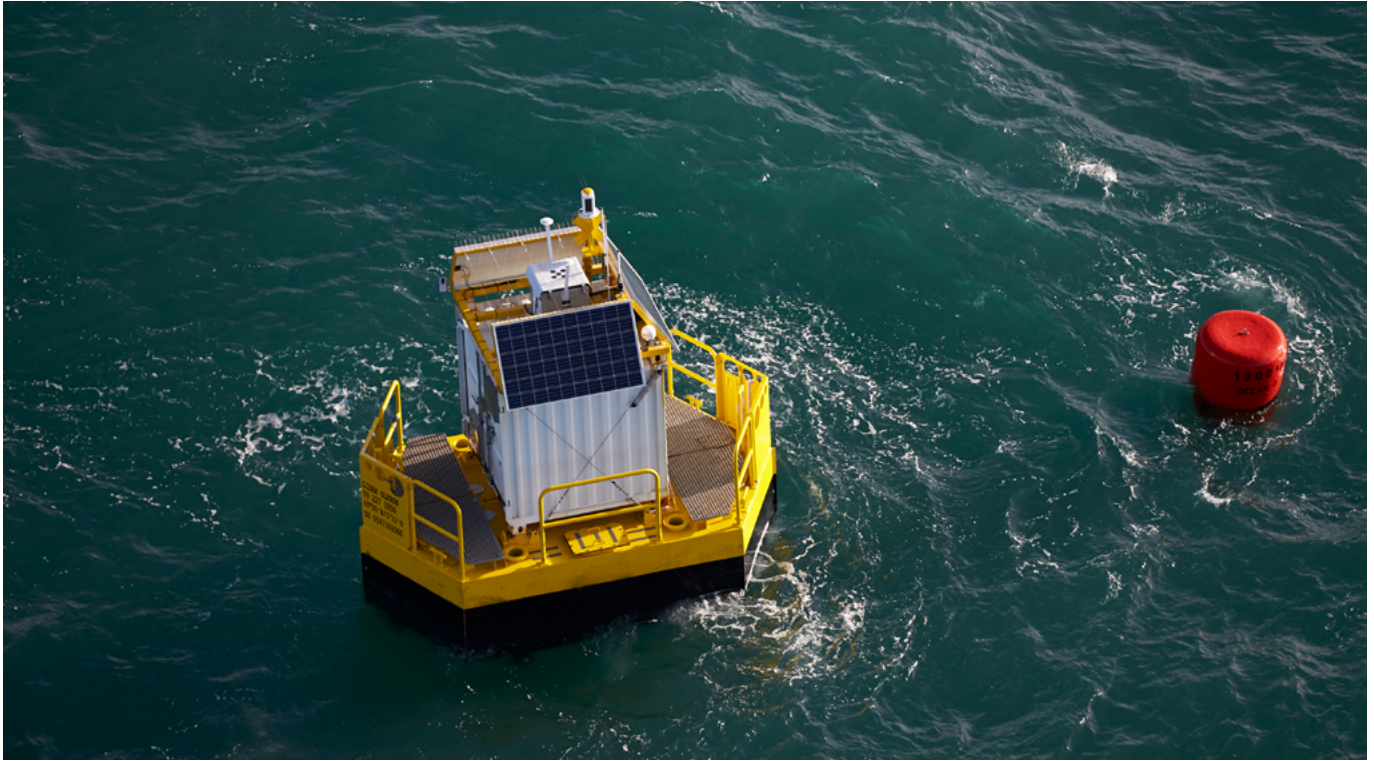
Figure 11: WindCube Offshore deployed on a buoy — The sunshade helps protect the lidar window against solar radiation, dejection, and splash in offshore deployments. Photo courtesy of Akrocean.
