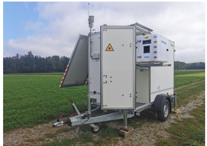
Figure 21: WindCube v2.1 and power supply solution integrated in a trailer — Photo courtesy of GWU.
