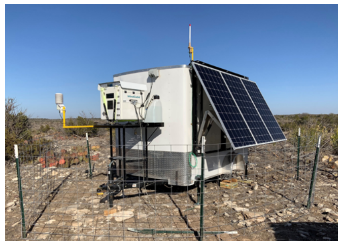
Figure 22: WindCube deployed with a solar PV + trailer solution to perform WRA in Texas, USA
