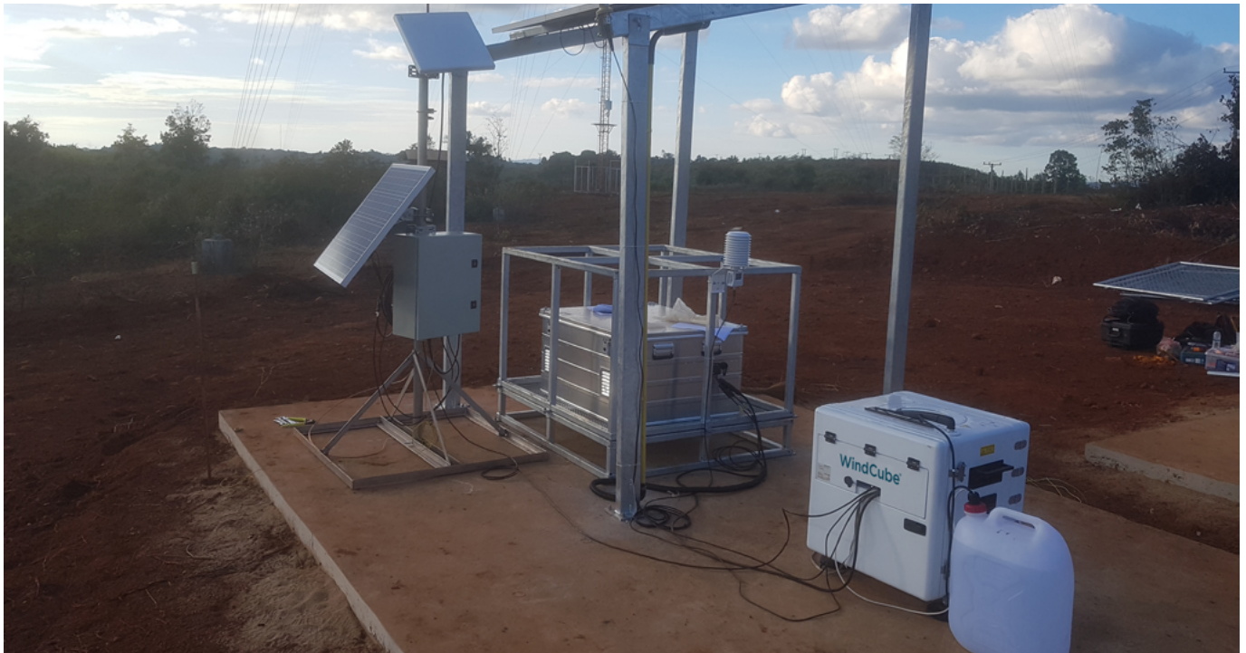
Figure 8: Example deployment adjacent to a met tower — Example deployment to perform WRA in Laos. The lidar is offset a few meters from outermost guy wire anchor. Beam CNR was closely checked during setup to confirm no guy wire interference. Photo courtesy of Impact Energy Asia Development Limited (IEAD).
