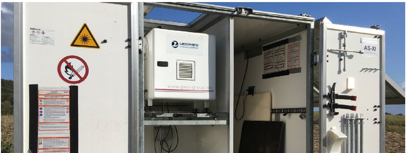
*Recent enhancements made to WindCube allows for 20 simultaneous heights and up to 300m.
